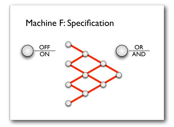
The four green buttons turn their nearby lamps on and off. The six red buttons are logic gates, collectively controlling the state of the lamp on the right. They behave as AND or OR gates. They are linked by the lines.
